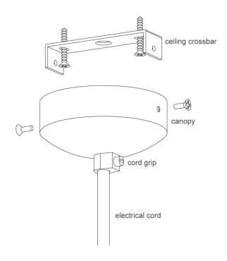
The light fixture is to be hanged from the matching white or black canopy set included in order, which is attached by screws to ceiling and then connected to existing electrical cord in ceiling. (Screws not included).
