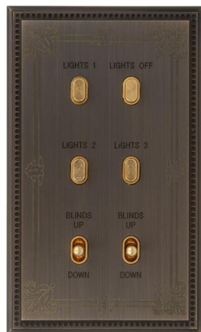
Solid brass, Bronze Médaille Foncé finish Machined and engraved edges 80x142x4 mm 4 Ellipse push buttons and 2 Seattle levers
