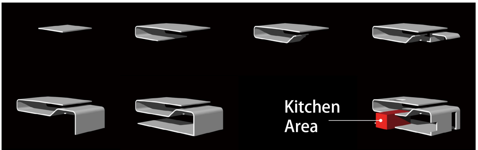
Animation showing the concept that a single plate is bent to become a floor / wall / ceiling
