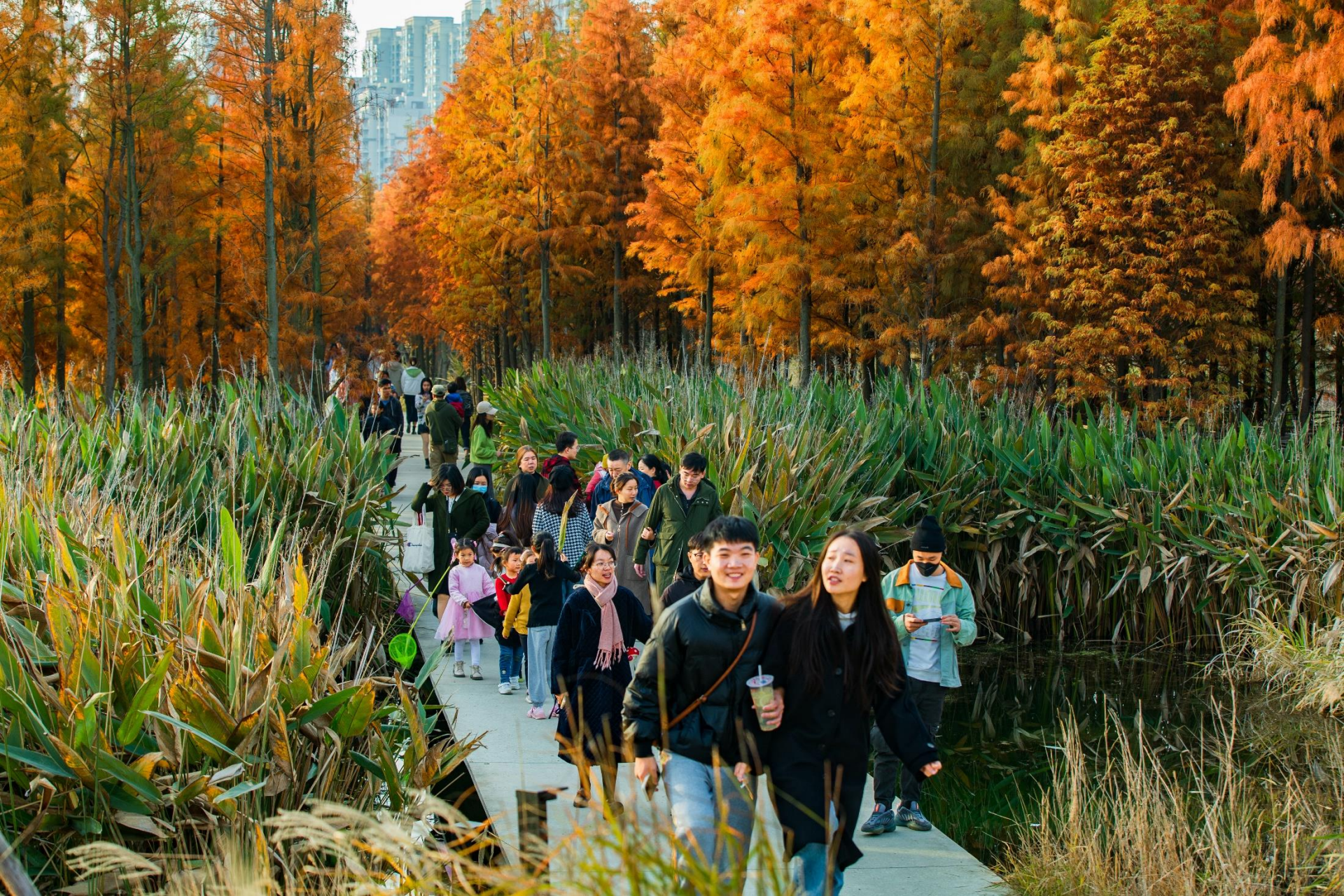
08. Visitors of all ages have embraced the opportunity for a new kind of immersive natural experience. The boardwalk and platforms are made of prefabricated concrete detached from ground so they can be easily washed clean after being submerged during flooding.
