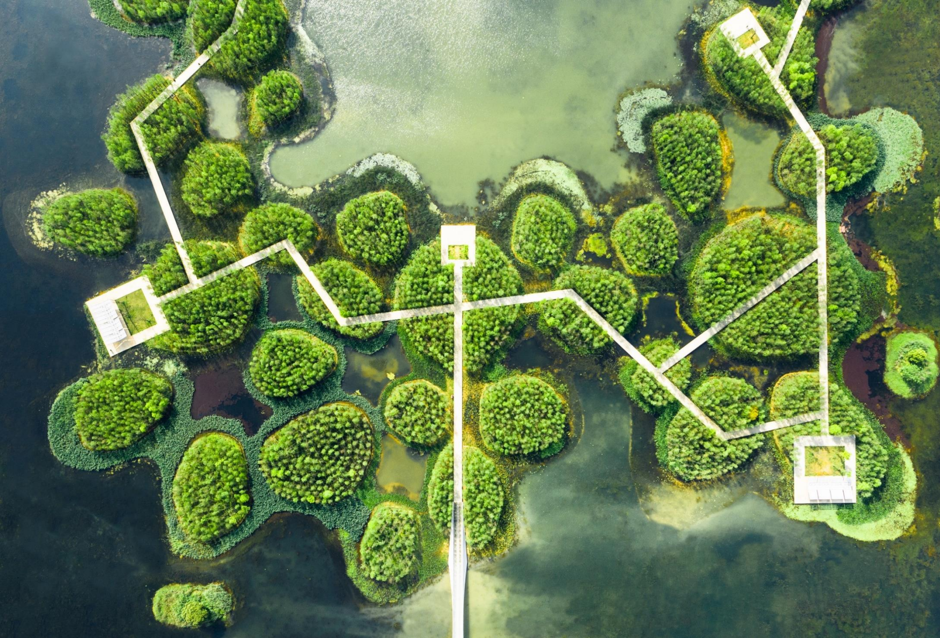
4. Inspired by the ancient concept of farming atop marshes, and Chinampa-style floating gardens, the coal ash dumped on the site was recycled and mixed with fill from the fish pond dykes to create a lake with numerous islets. 4
