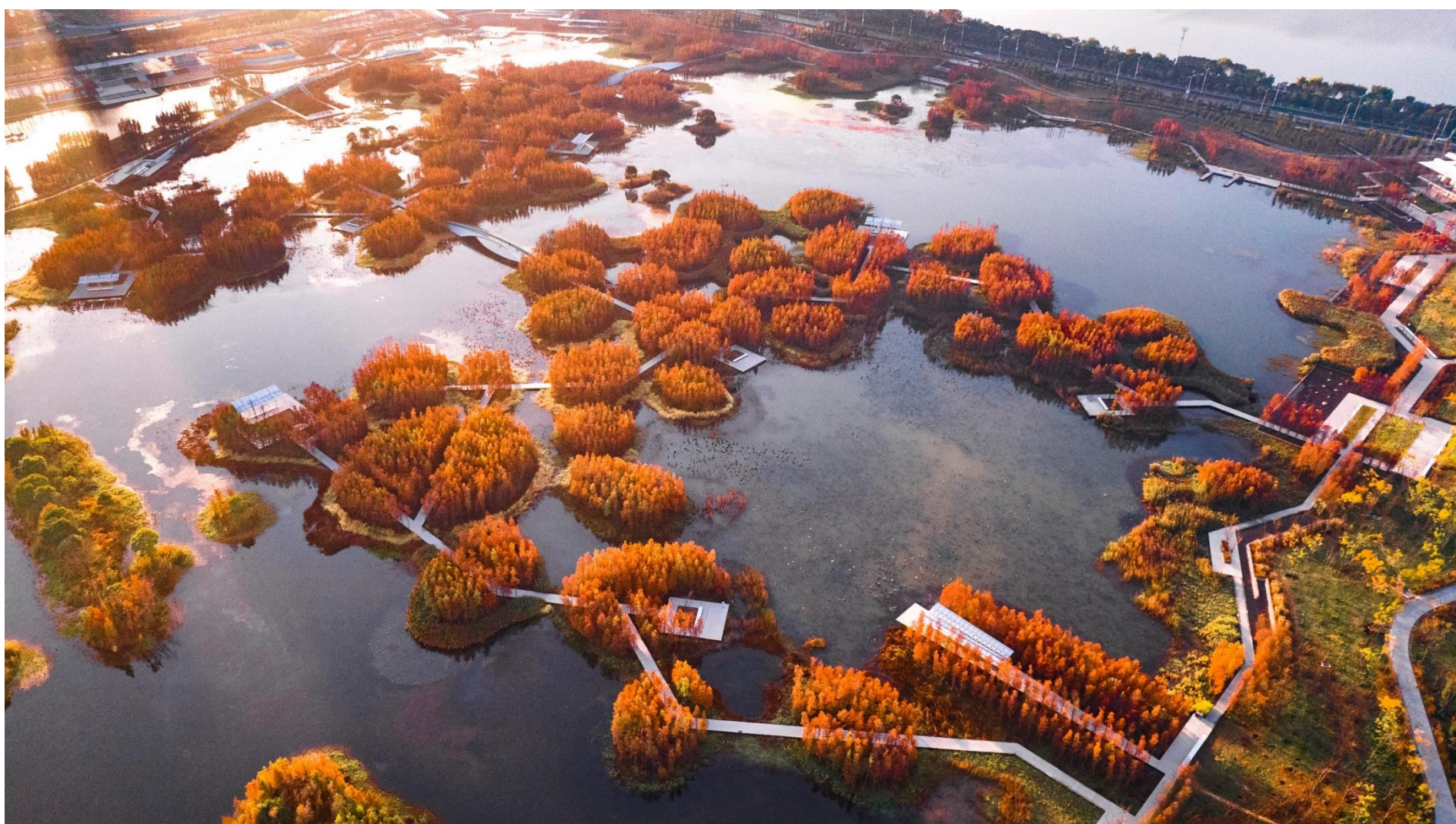
14 A bike route and service road follow the park's periphery. The waterfront at the periphery of the park, meanwhile, is designed to accommodate 20-year floods and provide a zone that can meet the recreational needs of the local population, and includes natural playgrounds, beaches, fountains and lawns.
