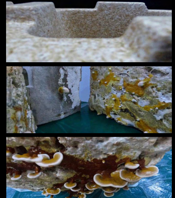
Mycelium Brick Manufacturing Process 菌丝砖出菇过程
