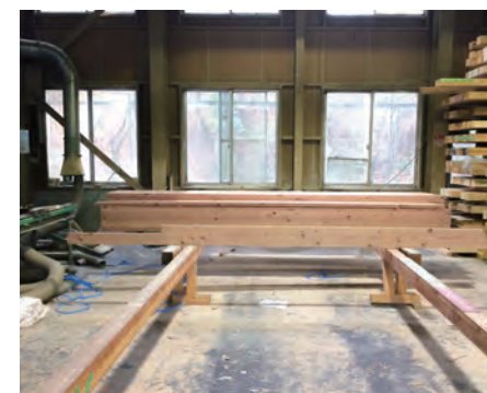
Pre-cut product inspection. A climbing rafter that is made of solid wood and cut inside and outside.
