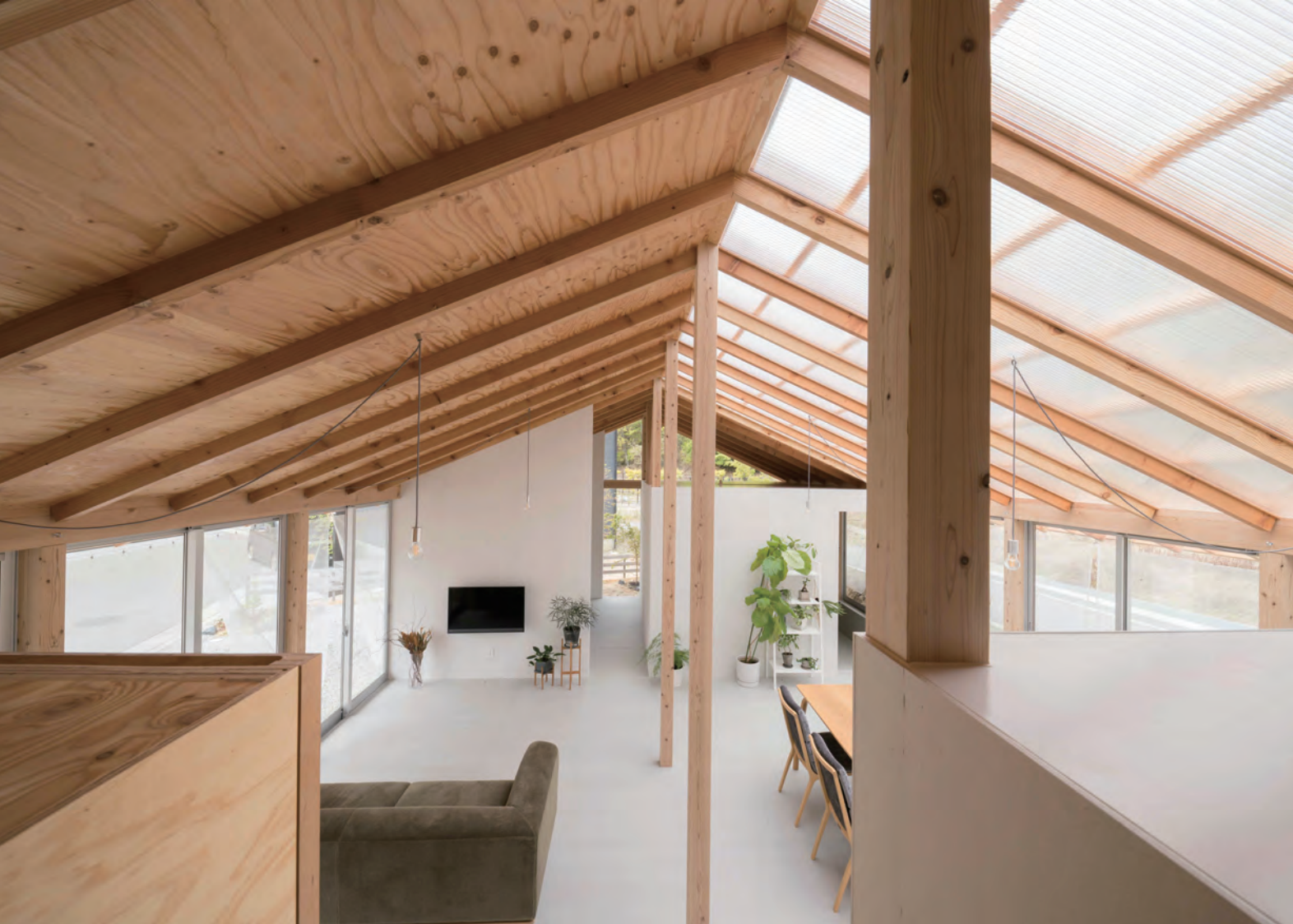
Living/dining kitchen. The space is 3.8m high and the space is gently divided by the two pillars and the wall. By using softwood plywood for ceilings, eaves, and fittings, and limiting the types of materials, we are trying to cope with
