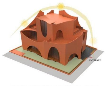
OPEN SPACES LIKE THE GARDEN AND DECK HAVE BEEN STRATEGICALLY PLACED IN THE NORTH OF THE SITE. THE SOUTH FACING FACADE HAS SMALLER SIZED ARCHED OPENINGS REDUCING HEAT GAIN
