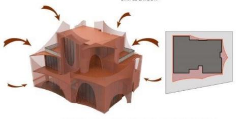
THE ADDITIONAL LAYER OF PUNCTURED SHEAR WALLS PROTECT THE INTERNAL VOLUMES FROM THE DESERT HEAT
