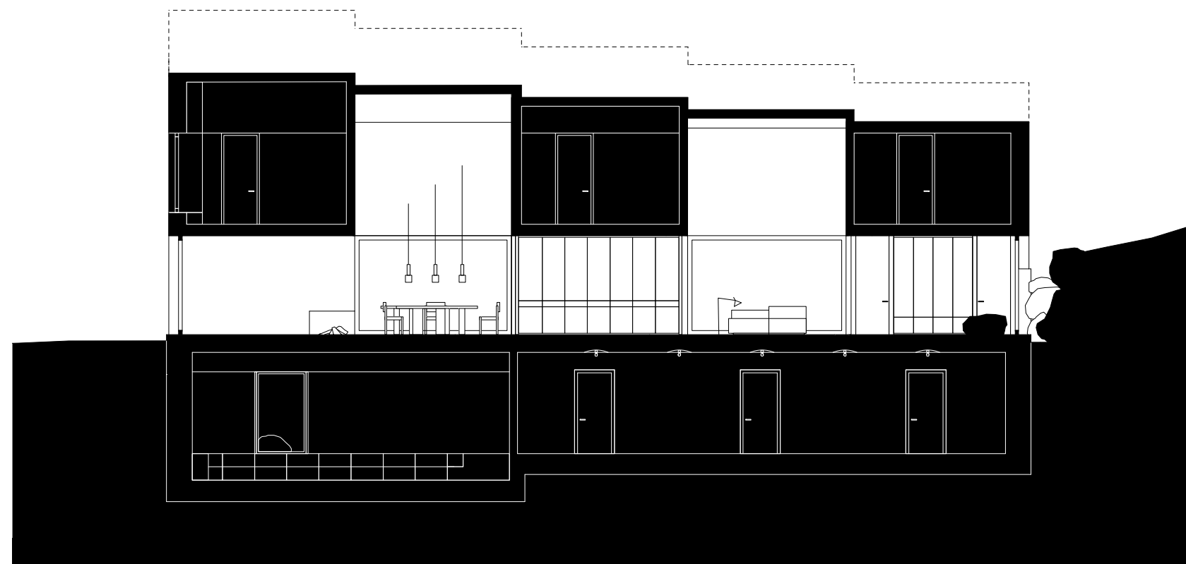
Section showing the basement with its corridor and miniature sports hall at the end.
