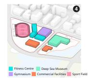
The fitness centre and the commercial facilities are relatively open and are placed on the west and south sides with better orientation and views. The gymnasium and the museum are relatively closed and are placed facing city inerface.
