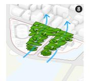
The large roof volume is broken into small parts and the corners are tilted so that the natural wind can enter the public space created by the roof of the interesting multi-functional threeterrace building, and at the same time, dimensional garden for the public. the tilted roof opens up the sea view for the lower buildings.
