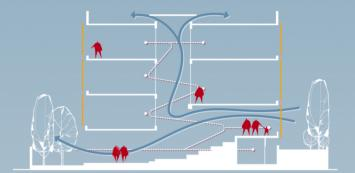
The Southern side of the site is raised in the form of a garden in order to harness the South breeze while also taking advantage of a wind channel caused by the extended road beyond the site. A spiral staircase comes out of the building face that leads up to a roof top cafeteria.
