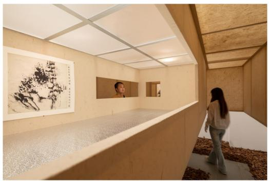
The whole installation is modularized at the scale of 640, and most of the components can be prefabricated off-site and assembled onsite, which improves the efficiency of the erection and reduces the disturbance of the construction to the site (library).
