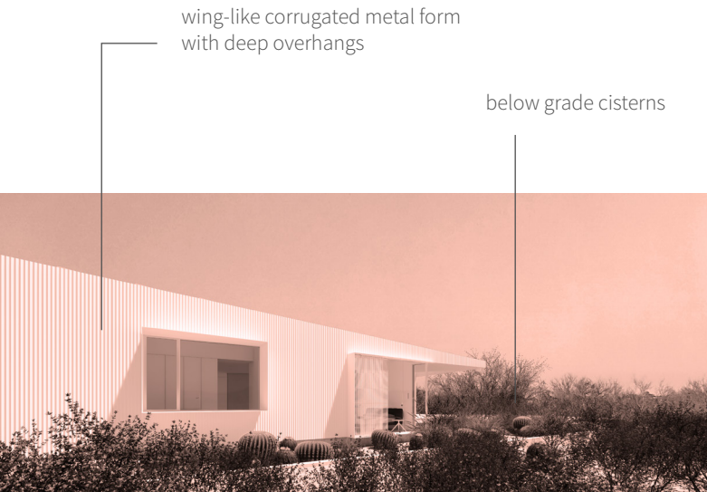
corrugated metal cladding on wood frame construction
